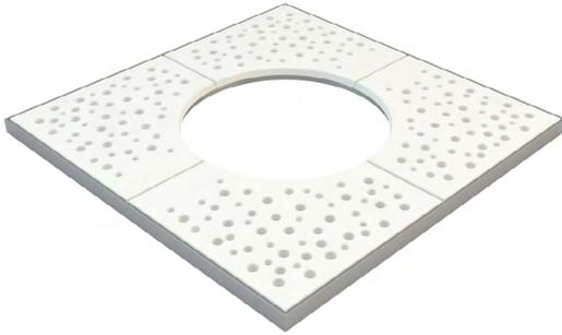
Description: Bubble Square plant protection grid, made of UTC (Ultra Tense Concrete), consisting of four elements with holes of different diameters to ensure the passage of water to the plant's root layer. Their alignment is guaranteed by means of a steel counterframe that will be cemented under the floor level.
